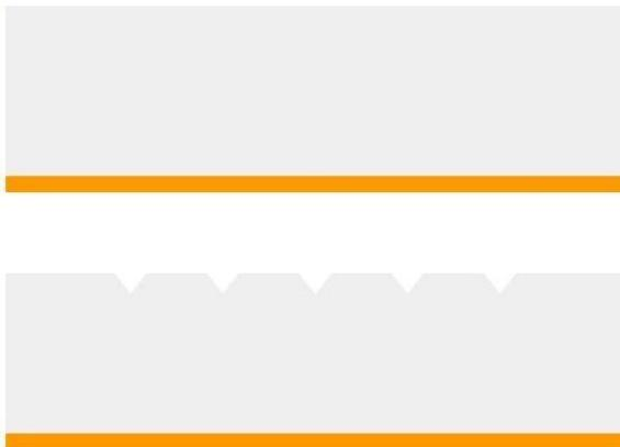
Figure 1 : (a) Opening of the front side oxide mask. (b) Front side alkaline etching. This leads to initiate the formation of non-through-silicon vias.
