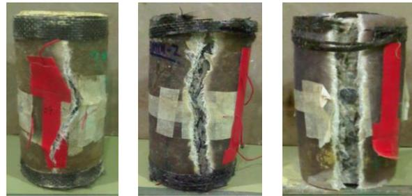
vertical rupture      partially inclined      inclined ruptures
