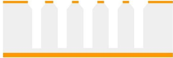
Figure 2: Deep Reactive Ion Etching leading to non-through-silicon vias.
