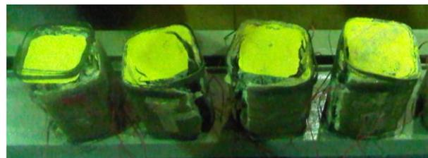
Figure 7: Failure mode of square specimens
