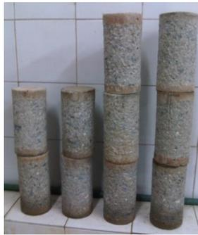
Figure 1: Typical roughened surface of specimens
