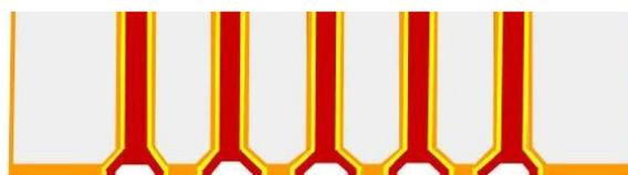
Figure 9: Backside Chemical Mechanical Polishing. This leads to the separation of through-silicon holes.
