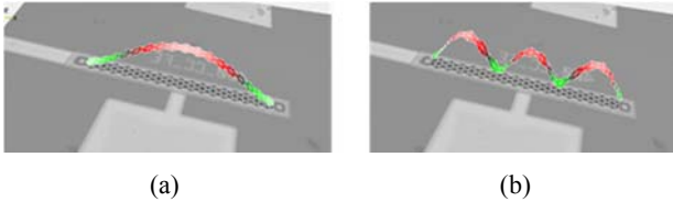
Figure 6: RMS values of the vibrational mode shapes of full electrode microbeam at (a) \omega_1 = 158.2 kHz, (b) \omega_3 = 729 kHz.
