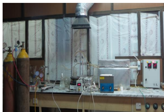
Figure (1) atmospheric pressure chemical vapor deposition system (APCVD)
