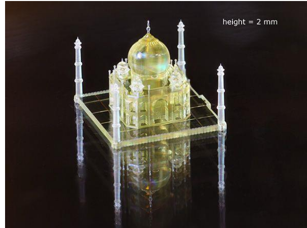
Figure 1: The Figure illustrates meso-scale printing with sub-micrometer feature sizes.
