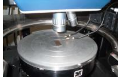
Figure 1. Experimental test on the perforated microplate with a laser vibrometer
