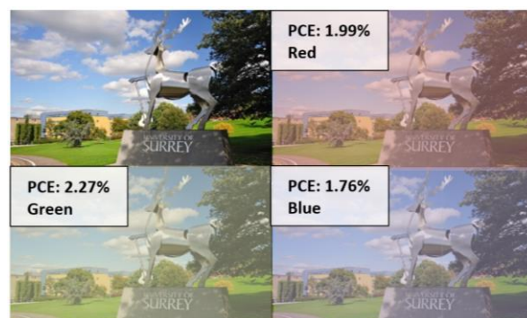
Figure 1: Illustrates different coloured semi-transparent OSCs (red, green and blue), all having an average transmissivity of 50%. The RGB values that have been used are Red (213, 148, 147), Green (200, 210, 172), and Blue (173, 182, 199). Each of the images shows the approximated power conversion efficiency for the materials used.
