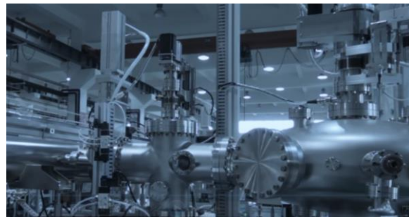
Figure 2: Picture of a corner of the vacuum-interconnected facility. Wafers could be transferred quickly by using automatically controlled cars in UHV tubes (pressure < 5 \times 10^{-8} Pa) between processing tools, avoiding any uncontrollable contaminations in air.
