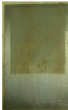
Figure 1: Epoxy coated sample undergone chalking after 72 hours of exposure to UV(B) radiation. Corrosion initiation in the effected area can be seen in the figure. The main aim of this work is to decrease the degradation due to weathering using nano Zinc oxide.
