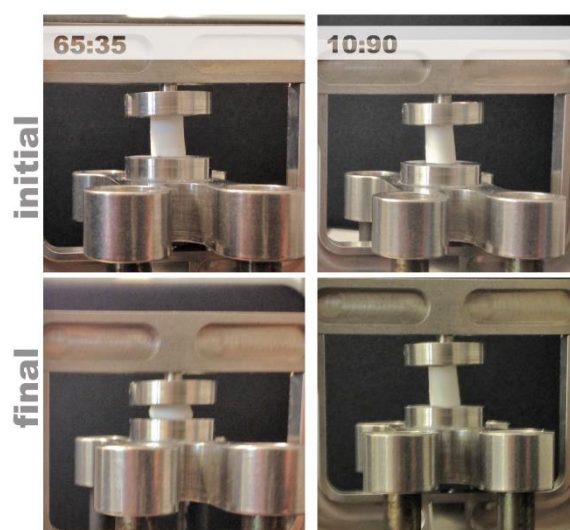
Figure 1: Photographs of two samples at the beginning and end of the compression test (force applied 18 N) with low (left) and high (right) amount of epoxy-resin.
