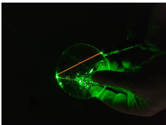
Figure 1: Figure illustrating a fluorescent photosensitive vitroceramic disk during laser irradiation.
