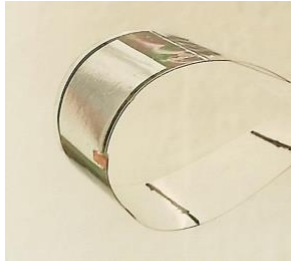
Figure 1: Photograph of flexible piezoelectric generator based on PZT thin film deposited onto an aluminium foil and encapsulated in a double PET sheet.
