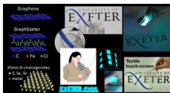
Figure 1: Figure illustrating different graphene and graphene related materials, i.e. few-layer graphene functionalized with FeCl 3 and metal di-chalcogenides. These materials are used to build devices for various electronics and optoelectronics applications such as flexible and wearable, transparent touch sensors, foldable light-emitting devices, and wearable, textile based light-emitting devices.
