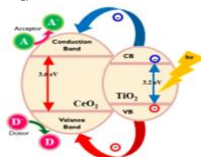
Figure 3. Mechanism of degradation of organics by CeO 2 -TiO 2 nanocomposite
