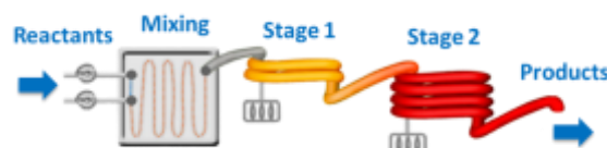
Figure 1: Figure illustrating the flow reactor system for large scale nanoparticles synthesis
