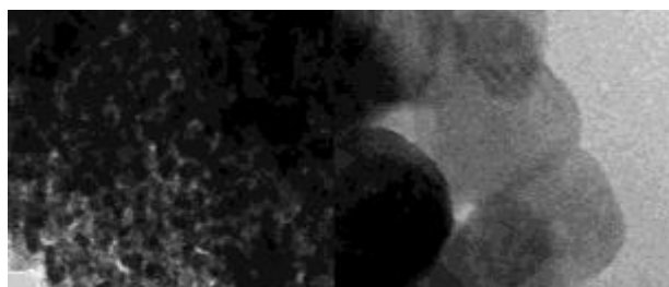
Figure 1: TEM images of mesoporous 2.0 % CeO 2 /TiO 2 nanocomposites (a) and HRTEM image (b)
