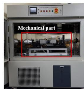
Figure 1: The test apparatus is located inside the environmental chamber which can change the temperature and humidity.
