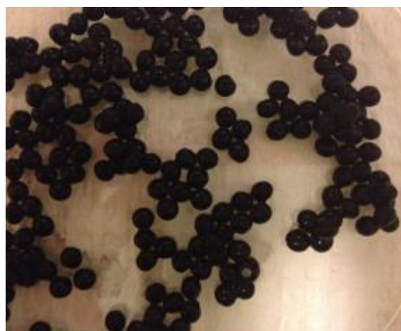
Figure 1: Top: silicon nanowire chip with 4 nanowire sensors made with in situ doped polysilicon [1]. Bottom: Alginate beads containing NZVIs. Each bead is 2mm in diameter [2].
