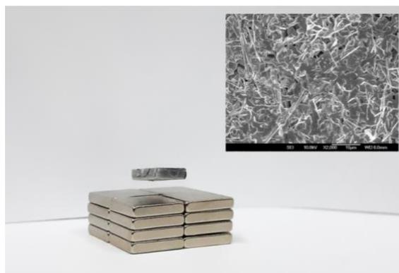
**Figure 1:** Meissner effect of the Bi-2212 superconducting sample at 300 Mpa with a thermal treatment at 840°C for 36 hours and its characteristic microstructure (SEM).
