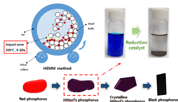
Figure 1: Synthesis experiment scheme of violet phosphorus as 2D material. It acts as a catalyst to reduce organic dye.
