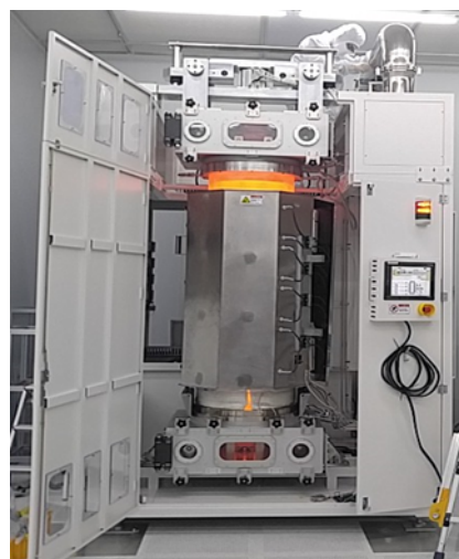
Figure 1: Roll-to-roll CVD system for graphene mass production.
