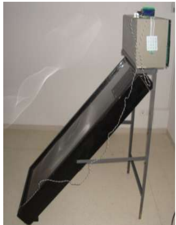
Figure 1: Photo illustrating the prototype of the proposed low cost solar dryer.
