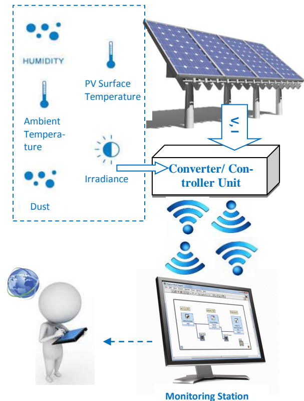
Figure 1: a general overview of the proposed wireless monitoring system. Sensors read various environmental parameters and the panel's current and voltage. These readings are sent to the controller unit where the readings are processed and sent wirelessly to the base monitoring station. The user can view and monitor the panel's performance from the web.
