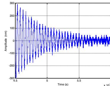
Figure 2. Displacement response of the perforated microplate
