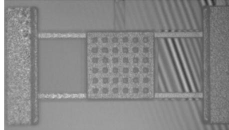
Figure 1. Optical image of the perforated microplate with four lateral elastic suspensions
