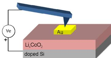
Figure1: Schematic view of an electrode/ $\text{Li}_x\text{CoO}_2$ /electrode device. A conducting AFM probe is in contact with the upper electrode. The bias is applied between the bottom electrode and the AFM tip.
