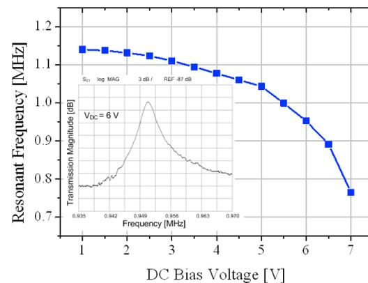
Figure 2: Measured resonant frequency versus DC tuning voltage. The inset shows two-port transmission frequency response magnitude plot.
