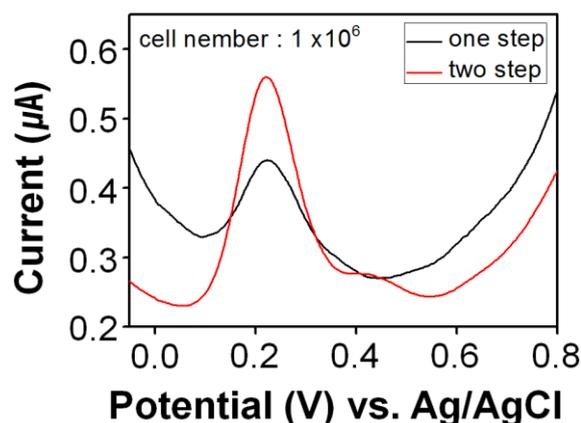
Figure 1: Comparison of sensitivity between 1- and 2-step O<sub>2</sub> plasma-treated SWCNT immunosensor : SWV of peak currents for 1- and 2-step O<sub>2</sub> plasma treated SWCNT electrodes following capture of CD4<sup>+</sup> T cells among  $1 \times 10^6$  splenocytes.
