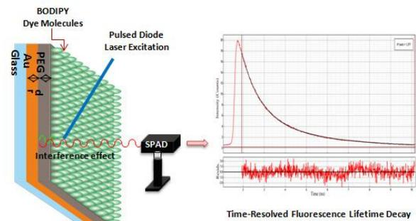
Figure 1: Figure illustrates humidity sensing mechanism based on the fluorescence lifetime of BODIPY dye molecules. The thickness of polymer layer changes the radiative decay rate of the dye molecules due to interference effect between emitted and reflected light waves.
