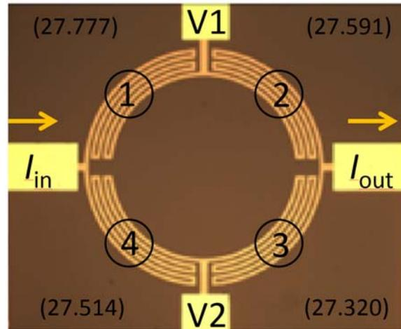
Figure 1: Ring sensor with information of thickness at the middle of the four arms, and the selection of current and voltage electrodes to minimize the voltage off-set
