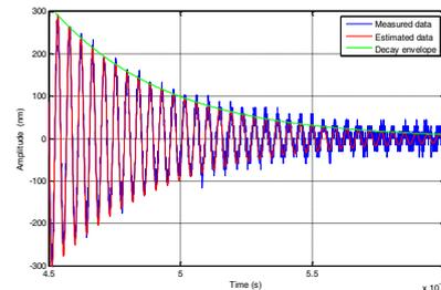
Figure 3. Comparison between the measured (in blue) and the reconstituted (in red) displacement response of the perforated microplate
