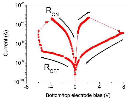
Figure 2: Typical  $I$ - $V$  characteristics of a device presented in Figure 1 (with a  $30 \times 30 \mu\text{m}^2$  upper electrode), exhibiting a resistive-switching behavior (sweeping rate of  $100 \text{ mV s}^{-1}$  from 0 to  $-6 \text{ V}$ , back to  $+8 \text{ V}$ , and ultimately to  $0 \text{ V}$ ). In this example, the  $R_{\text{OFF}}/R_{\text{ON}}$  ratio reaches  $3 \times 10^3$  (measured at  $+1 \text{ V}$ ).
