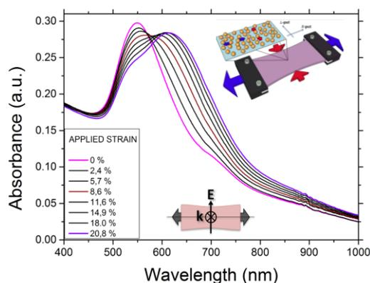
Fig. 1: In the figure is shown the development of plasmonic coupling with the increasing of mechanical strain of sample.
