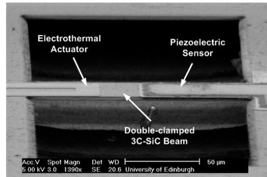
Figure 1: SEM of the fabricated resonator with the u-shape layout of the electrothermal actuator (input port) and piezoelectric sensor (output port) placed on the top of 3C-SiC double-clamped beam.
