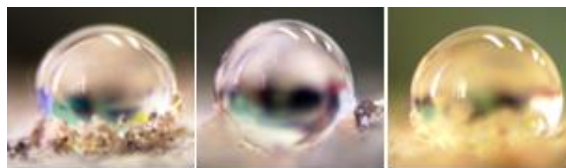
Figure 1: Water droplet at the surface of hydrophobic material with a contact angle of 157^\circ .
