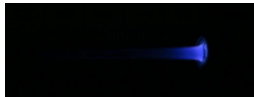
Figure 2: Photo of the argon-based non-thermal atmospheric pressure plasma jet ( V = 10 kV; f = 10 kHz).
