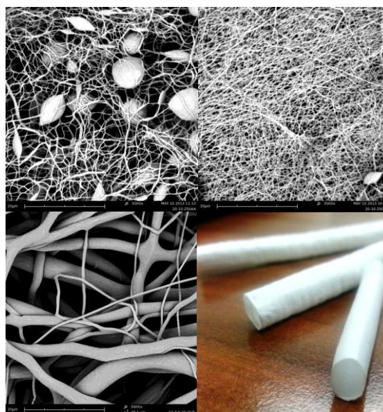
Figure 1: Morphological analysis of PCL (a-c; scale bars: 5000X) scaffolds based on the use of different solvent systems as acetic acid (a), formic acid (b); and chloroform:ethanol (c). Macroscopic picture of PCL tubular scaffolds (d) .
