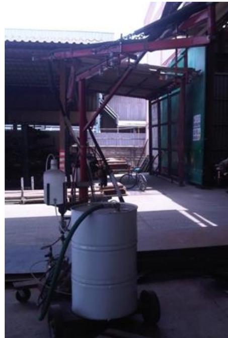
Figure 1: Figure showing the pumping and spraying equipment for sprayed glass fiber reinforced polymer composites (SGFRP).
