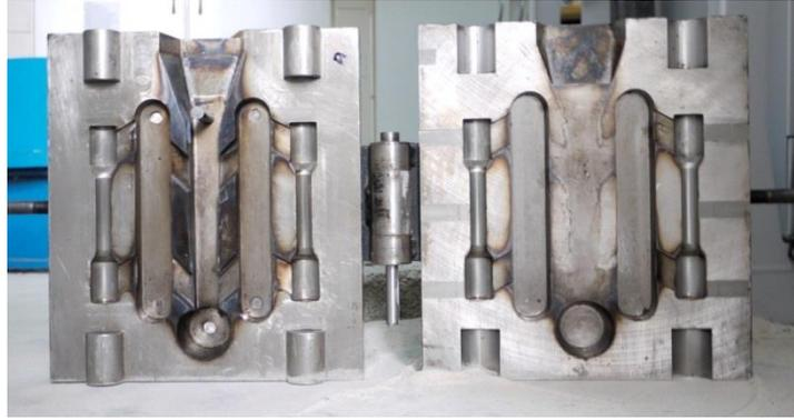
Fig. 1 Core and cavity of die
