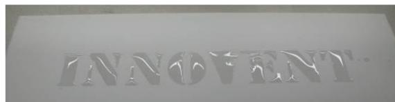
**Figure 1:** local hydrophil/hydrophob surface functionalization preparing antibacterial and easy-to-clean properties.
