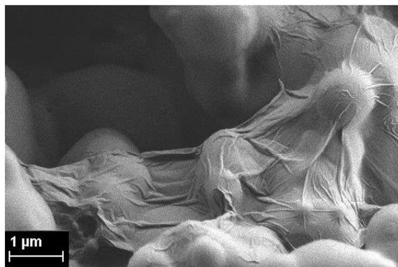
**Figure 1:** SEM images of the PVC spheres covered with the GO sheets.
