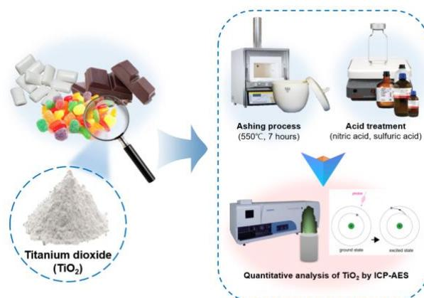
**Figure 1:** Schematic illustration for quantitative analysis of TiO<sub>2</sub> by ICP-AES after pretreatment such as ashing process and acid treatment.
