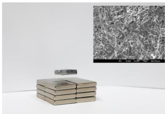
**Figure 1:** Meissner effect of the Bi-2212 superconducting sample at 300 Mpa with a thermal treatment at 840°C for 36 hours and its characteristic microstructure (SEM).
