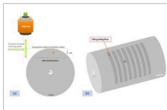
**Figure 1.** Illustration of an optical fiber micromachined to write an external sensing structure.
