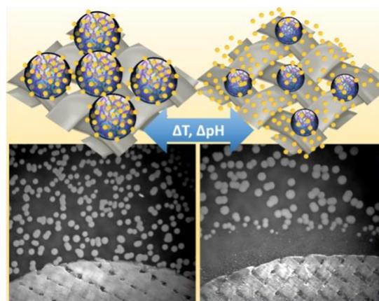
**Figure 1:** Pro-active release of antimicrobials from the poly-(N-isopropylacrylamide) / chitosan (PNCS) hydrogel functionalised textile substrate upon the shrinking of the hydrogel particles.
