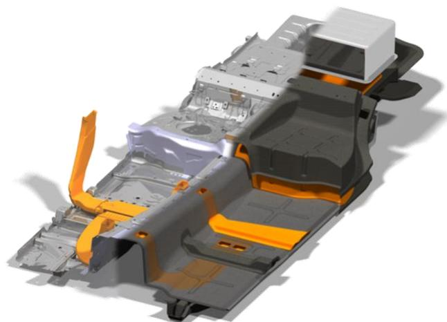
**Figure 1:** LeiFu (Lightweight with integrated functionalities) - Automotive CFRP underbody structure
