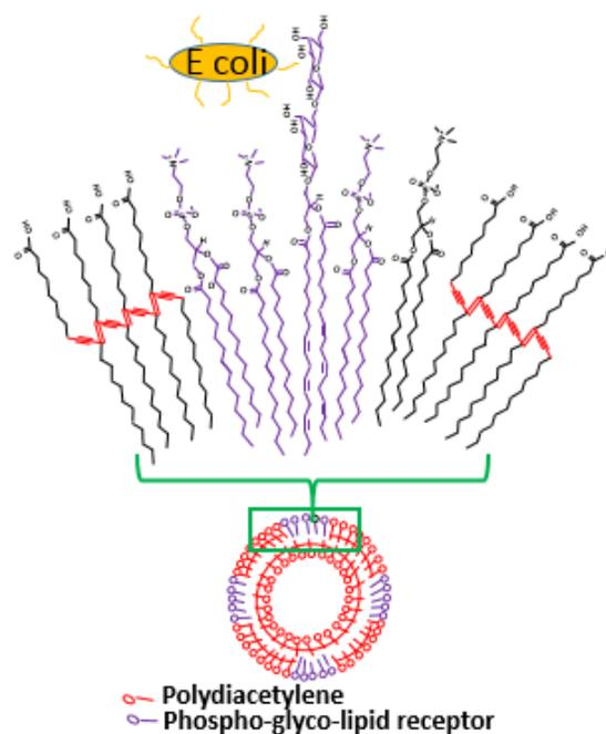
**Figure 1:** Schematic diagram of a polymerized vesicle composed of polydiacetylene and a specific phospho-glyco-lipid recognition receptor for E.coli. Once the E. Coli is attached to the receptor, a color transition from blue to red is observed.
