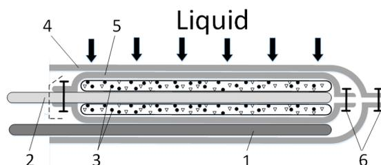
**Figure 1:** Flexible textile Al-Air battery cell
