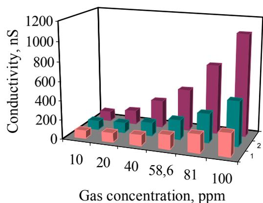
**Figure 1:** Typical conductivity dependence of  $\text{Mn}_3\text{P}_2\text{Mo}_{18}\text{O}_{62}$ -silica film on gas concentration in air: 1 - water vapours, 2 – ammonia, 3 – ethanolamine.
