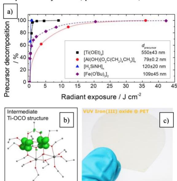
**Figure 1:** a) Comparison of VUV-induced (Xe-excimer irradiation;  $E_{\text{photon}} \approx 7.2\text{ eV}$ ) decomposition of different coordination compound thin films on Si-wafers depending on the applied radiant exposure ( $H_e$ ) at ambient conditions. b) Structure of an intermediate  $\text{Ti}(\text{OCO})$  ring structure from DFT calculations. c) SEM image of a VUV-irradiated PET substrate showing a crack-free metal oxide coating.
