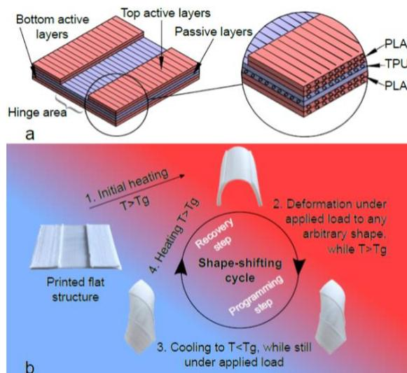
**Figure 1:** Figure illustrating the fundamental principle of 4D-printed, morphing structures
