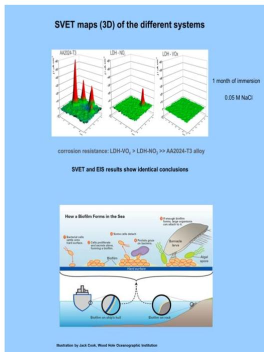
**Figure 1.** SVET maps of AA2024 alloy in NaCl solution and in presence of inhibitor containing LDH (upper part) and biofilm formation in seawater (lower part).
