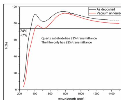
**Figure 3:** Transmittance spectra for as deposited sample at 250°C vacuum annealed sample at 400°C.
