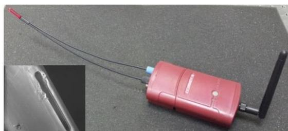
**Figure 1:** Polymer fiber optic sensor integrated in an autonomous wireless sensing node. Inset, presents a micromachined optical sensing head.
