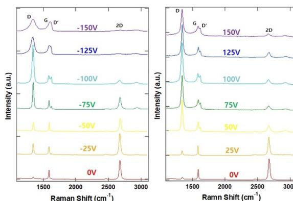
**Figure 1:** Raman spectrum of Hydrogenated graphene applied back gate voltage from -150 V to +150 V during hydrogen plasma treatment
