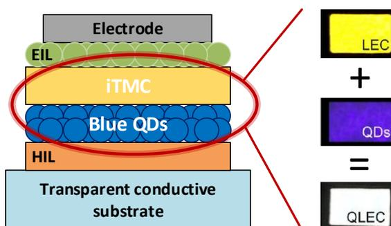
**Figure 1:** Figure illustrating the device concept of a hybrid QLEC (based on Frohleiks et al., 2018). The idea is to combine the high-performing yellow-orange emitting iTMC-LEC with blue quantum dots to generate bright white light with high CRI.
