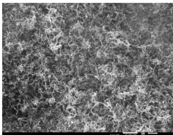
**Figure 1:** Scanning electron microscopy (SEM) micrographs for carbon nanotube morphology obtained by impinging flame.
