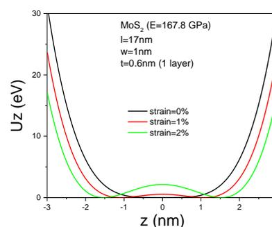
**Figure 1:** Elastic energy vs. out-of-plane displacement ( $z$ ) for different compressive strain values of a  $17 \times 1 \times 0.35$  nm<sup>3</sup> MoS<sub>2</sub> ribbon.
