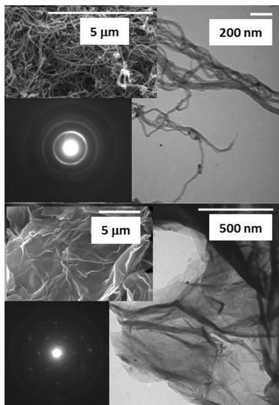
**Figure 1:** Figure shows typical TEM, SEM images, and electron diffraction patterns (EDP) of MWCNT and rGO.
