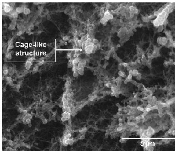
**Figure 1:** SEM micrographs of PE/modified VACNTs. This SEM micrographs shows the cage-like structure obtained by joining carbon nanotubes tips coated with a polymer layer.
