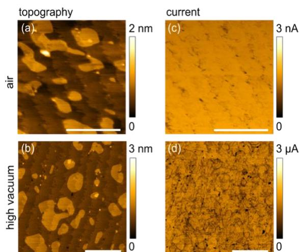
**Figure 1:** cAFM from the same 3-4 layered MoS<sub>2</sub> sample showing the increased current level and sensitivity under high vacuum. (a) and (b) Topography (c) current images in air at 5 V bias (d) current images taken immediately after pumping to high vacuum at 0.5 V bias. The data taken in air and high vacuum was acquired using identical parameters: same probe with spring constant  $k$  of 7 N/m, set point of 10 nN, and 1 Hz scan rate. Scale bar is 500 nm.
