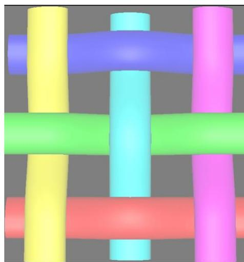
**Figure 1:** 3D model of a woven structure with different colours indicating yarns with different properties, for example actuation ability. Locking certain yarns and letting others move freely for example by open yarn spacing enables overall movement of the so formed fabric.
