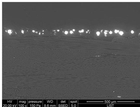
**Figure 1:** Figure illustrating a copper coating on a functionalized CFRP substrate
