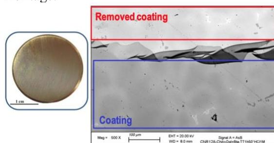
**Figure 1:** Optical and SEM images of Cu-based alloy substrate coated with chitosan-based protective coating after thermal treatment (1 h, 50 °C) with acid vapours. In the SEM image the boundary between the film and the bare alloy after film removal can be appreciated.
