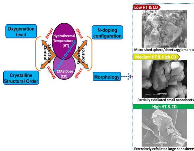
**Figure 1:** Controlled synthesis of NG with tuned structural features.
