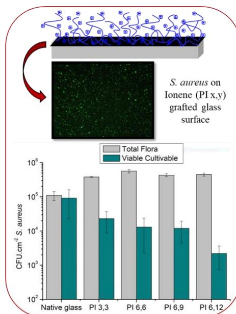
**Figure 1:** Upper : Epifluorescence microscopy of fluorescent *S. aureus* strains (total flora) on ionene surfaces. Lower : Enumeration of viable cultivable bacteria and total adherent bacteria of *S. aureus* strains in the presence of initial glass substrate and ionene surfaces.
