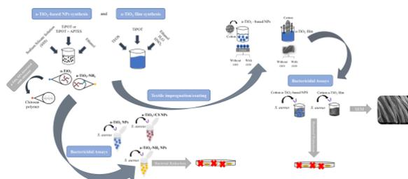
**Figure 1:** Schematic of a-TiO<sub>2</sub> based nanoparticles synthesis, textiles impregnation/coating and nanoparticles/films/textiles bactericidal performance evaluation.
