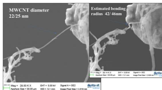
**Figure 1:** Illustration of the gripping and bending of a single 30 nm diameter MWCNT, in the  $\mu$ Robotex facility of the FEMTO-ST institute.
