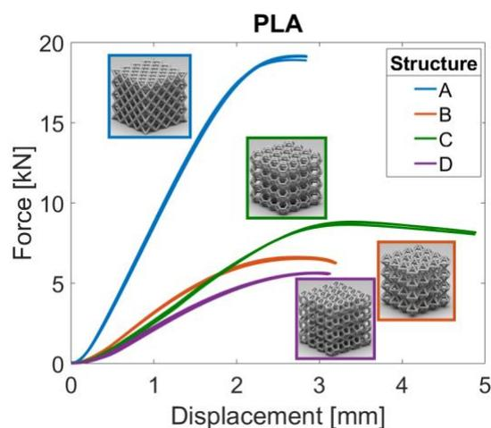
**Figure 1:** Mechanical properties of different PLA structures printed with fused filament fabrication - the figure shows the curves of the compression tests until the point of ultimate compressive strength.
