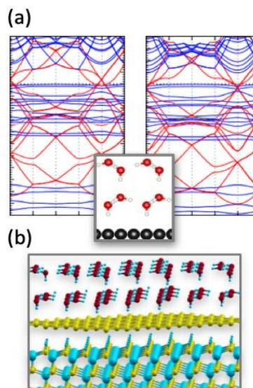
**Figure 1:** (a) bandstructures of 2ML ice on graphene. Adsorbate orientation and application of static electric fields lead to *p*-type and *n*-type doping. (b) substrates with different lattice mismatches affect doping. On SiC, water mediated *n*-type doping survives, while *p*-type doping is suppressed.
