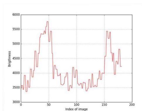
**Figure 2:** Brightness of the region of bending with respect to the index of image in the sequence of images: peaks of brightness correspond to maximum of bending.
