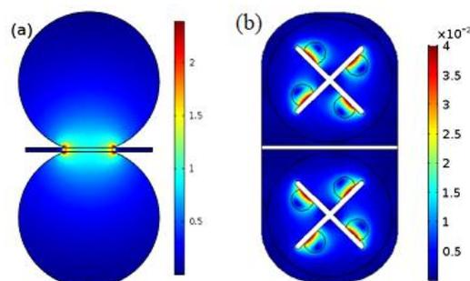
**Figure 1:** The current density distribution due to electronic charge transfer to electrode phase in two different geometries. (a) Static slurry while charging, (b) Mixing slurry while charging.
