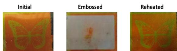
**Figure 1:** Example of time-temperature dependent camouflaging of a printed pattern.
