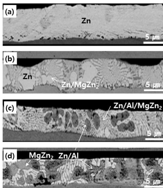
**Figure 1:** Figure shows a picture of the FE-SEM cross section of the Zn-Al-Mg alloy layer with the variation of Al and Mg composition. Various intermetallic compounds such as MgZn<sub>2</sub>, Zn/MgZn<sub>2</sub>, Zn/Al and Zn/Al/MgZn<sub>2</sub> were formed within the coating layers.
