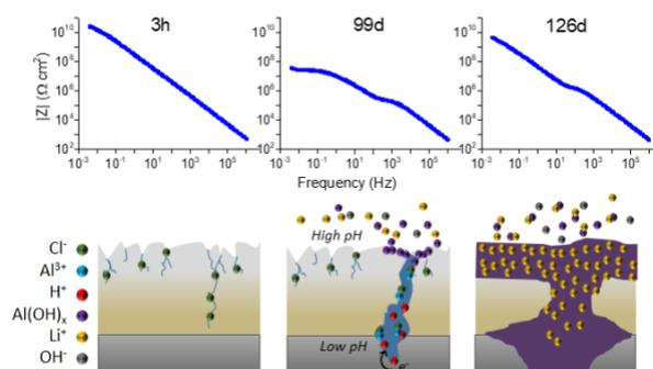
**Figure 1:** Time evolution of the impedance modulus of the PMMA-silica coating containing 1000 ppm of Li immersed in 3.5% NaCl along with the proposed self-healing mechanism for the formation a protective barrier.
