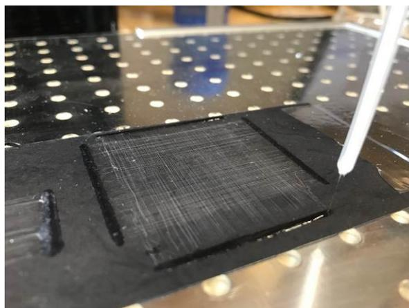
**Figure 1:** Scaffold made using drawing method.
