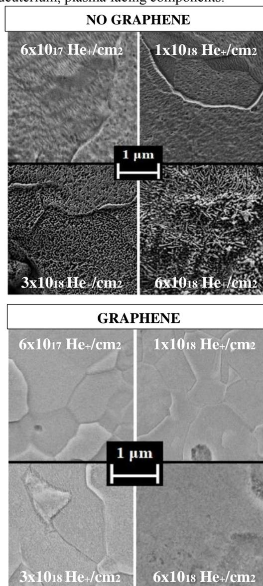
**Figure 1:** Surface morphology changes to the tungsten under intense helium irradiation at 30 keV, 900 °C.
