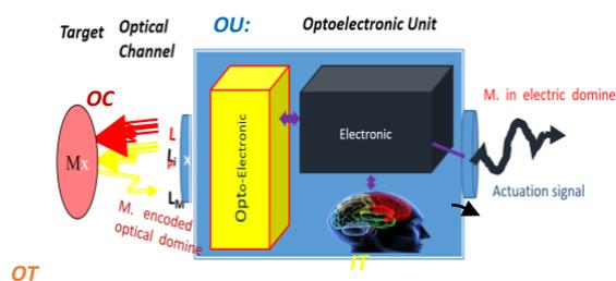
**Figure 1:** .- Illustration of a general Smart Light based Sensor system architecture: optical transducer on the target (OT); optical channel(OC); optoelectronic unit (OU); intelligence (IT).
