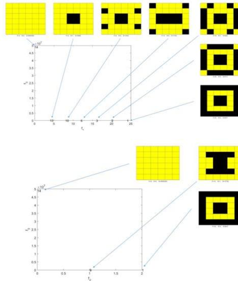
**Figure 1:** Figure illustrating the multiobjective solutions for optimal placement of sensors and actuators on the surface of a viscoelastic sandwich plate in order to minimize sound radiation, added mass and number of controllers.
