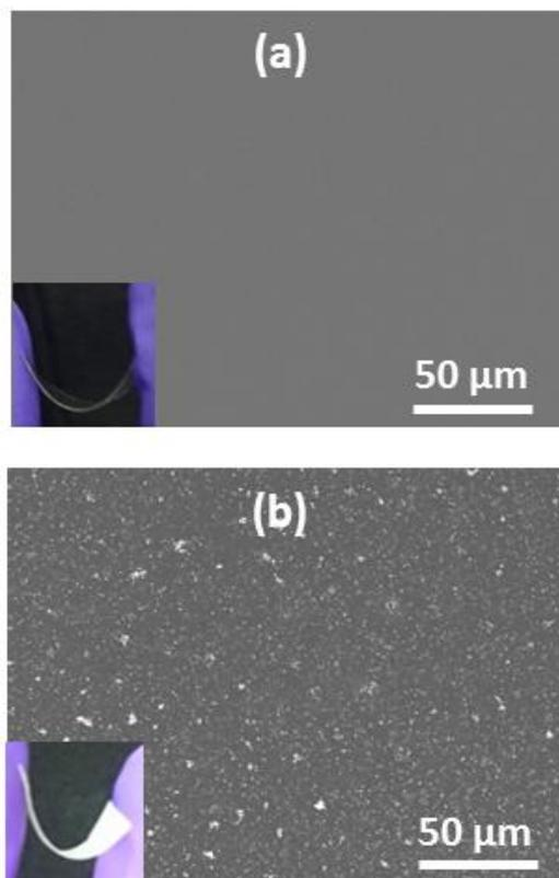
**Figure 1:** SEM images of surfaces of (a) neat PVA film and (b) composite film with 10 vol% BT 200 nm content. Insets: photographs of the films highlighting their flexibility.
