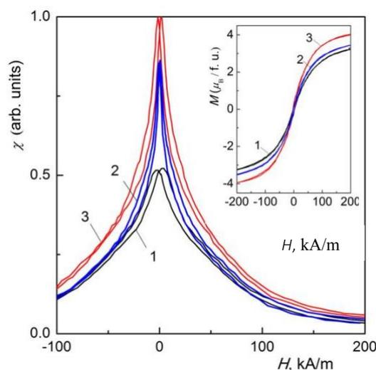
**Figure 1:** Magnetic field-dependent AC magnetic susceptibility  $\chi \sim dM/dH$  and magnetisation,  $M$ , measured at RT for Co<sub>2</sub>MnSi/Si(001) films annealed in vacuum at  $450^\circ\text{C}$  for 0.5 h (1), 1.5 h (2) and 4.0 h (3)
