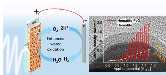
**Figure 1:** (left) Diagram illustrating the use of photoanodes for water oxidation, the bottleneck reaction in water splitting for hydrogen generation. (right) TEM image of  $\alpha$ -Fe<sub>2</sub>O<sub>3</sub> and FeO<sub>x</sub> amorphous coating and photocurrent results.
