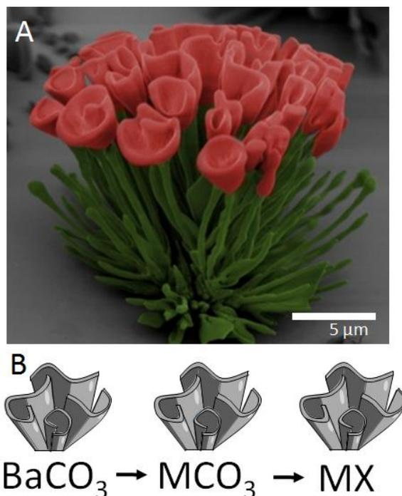
**Figure 1:** A. Example of a microshape. B. Schematic showing how microshapes can be transformed from their original composition towards a large variety of compositions.
