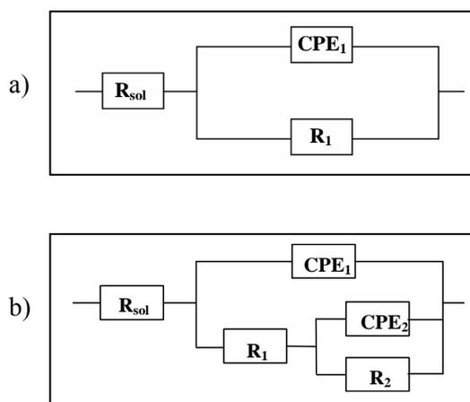
**Figure 1:** Figure illustrating the equivalent circuits used for the fitting of the experimental data where  $R_{\text{sol}}$  is the ohmic resistance of the electrolyte. a) The first circuit has one time constant.
