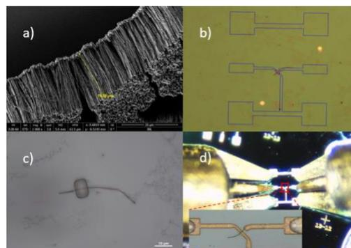
**Figure 1:** a) Grown nanowires attached to the seed layer. Scale bar:  $20\ \mu\text{m}$ . b) AutoCAD masks for the devices. c) Lithography of the graphene channel. Scale bar:  $10\ \mu\text{m}$ . d) Contact between the RF probes and the pads of the RF device. Inset showing a close view of the core-shell Ni/NiO nanowire and the self-aligned Drain-Source contacts.
