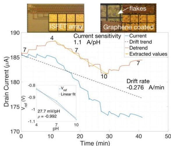
**Figure 1:** Plain ISFET arrays (top left) and multilayer graphene coated ISFET arrays (top right). The plot shows the real-time effect of drift on the drain current measurement while changing the pH of the electrolyte solution. The drift can be corrected in software to enable the real calculation of the pH sensitivity. Inset shows the sensitivity in terms of mV/pH. s
