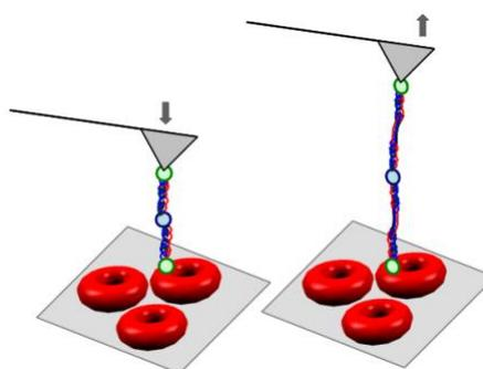
**Figure 1:** Schematic representation of the measurement by AFM-based force spectroscopy of the force necessary to overcome the fibrinogen-erythrocyte binding.
