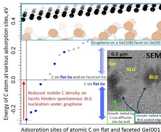
**Figure 1:** Growth-induced faceting of Ge(001). **Plot:** C atom energy at various sites on flat (blue) and faceted (gray) surface. **SEM:** Single-layer graphene (SLG) with parasitic bi-layer (BLG) islands; flat area is uncovered Ge. Faceting and BLG formation are explained by DFT results.
