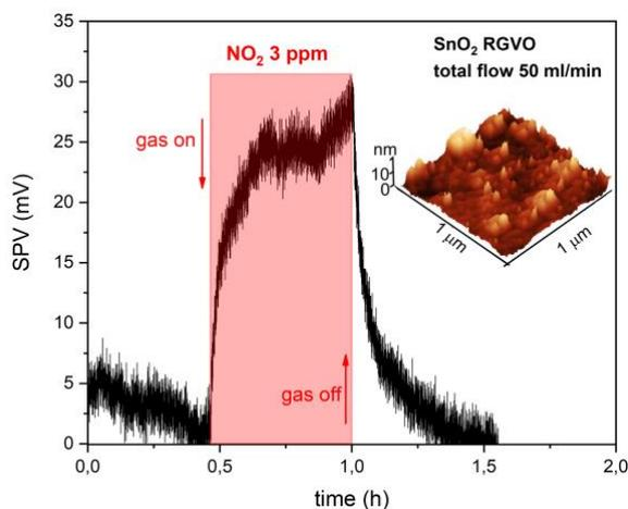
**Figure 1:** Gas sensor response of SnO<sub>2</sub> RGVO thin film towards 3 ppm NO<sub>2</sub>; SPV denotes surface photovoltage; the inset: AFM image presenting morphology of the sample.
