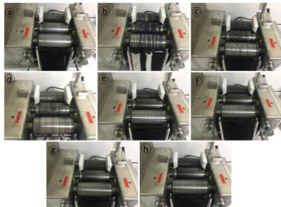
**Figure 2:** Three roll mixing process of 1.2 wt. % MWCNT-COOH and 400 g epoxy; a) first cycle-beginning at 3 min of endurance at 20 rpm, b) first cycle-finish with 23 min endurance at 20 rpm, c) second cycle with 23 min endurance at 20 rpm, d) third cycle with 16 min endurance at 25 rpm, e) fourth cycle with 16 min endurance at 25 rpm, f) fifth cycle with 13 min endurance at 28 rpm, g) sixth cycle with 12 min endurance at 30 rpm, h) seventh cycle with 10 min endurance at 35 rpm
