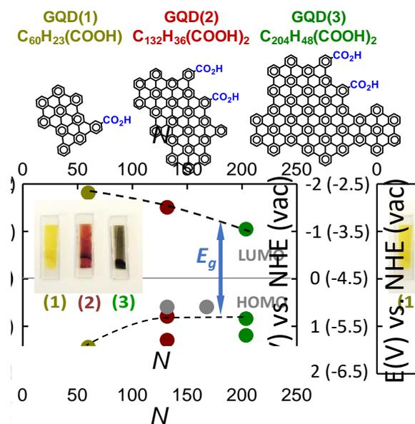
**Figure 1:** Examples of GQDs prepared by a “bottom up” surface-assisted synthesis approach and the experimentally determined dependence of the electronic structure on their size. The inset shows a photograph of the films with GQDs adsorbed on a transparent glass substrate.
