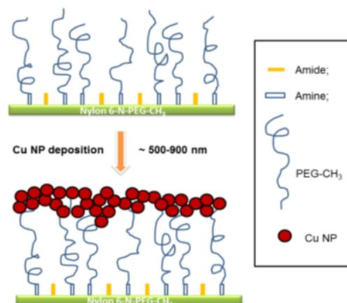
**Figure 1:** The conversion of Nylon 6 into Nylon 6-NH, followed by grafting on Nylon 6-NH via H<sub>3</sub>C-PEG-OTs and Cu NPs to form Nylon 6-N-PEG-CH<sub>3</sub>-Cu.
