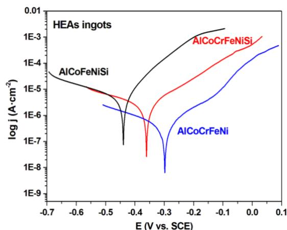
**Figure 1:** Polarization curves of selected HEAs tested in 3.5% NaCl solution at 25°C. The AlCoCrFeNi alloy exhibits the best corrosion potential which is shifted towards positive values.
