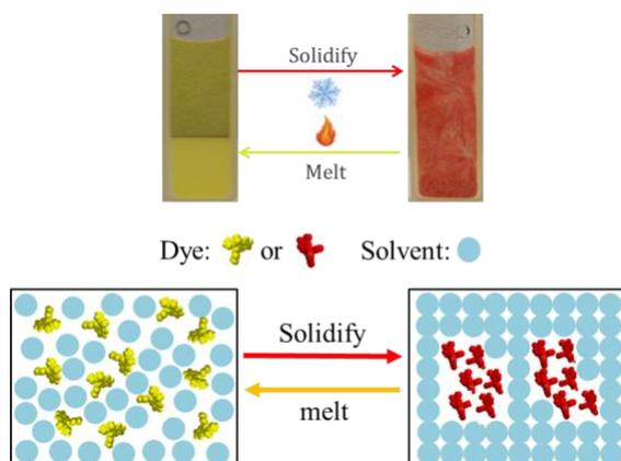
**Figure 1:** The photographic images of dye-solvent binary system that shows clear reversible thermochromism between liquid and solid states. The corresponding schematic diagram illustrates the colour change mechanism of solubility-dependent  $\pi$ - $\pi$  stacked agglomeration or disagglomeration of sulfonephthalein dyes controlled by melting or crystallisation processing of the solvent.
