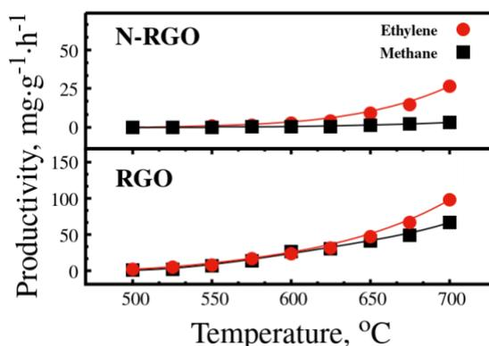
**Figure 1:** Dependences of ethylene and methane formation productivity on temperature for N-RGO and RGO. Productivity dimensionality is mass of products in “mg” per 1g of the catalyst per 1 hour. Catalyst load is 500mg. The inlet gas mixture flow rate is 10 ml/min with helium-to-ethane ratio of 1:1.
