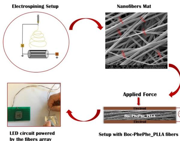
**Figure 1:** Electrospinning setup; SEM images at high magnification level (50,000x) of Boc-PhePhe\_PLLA electrospun fibers; Schematic piezoelectric setup with Boc-PhePhe\_PLLA fibers mat and LED circuit powered by the fibers array.
