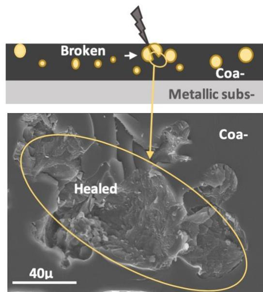
**Figure 1:** Schematic of coating containing microcapsules, and SEM image of polymerized microcapsules under the damaged zone of the coating.
