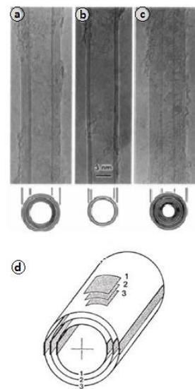
**Figure 1:** Electron micrographs of microtubules of graphitic carbon a) 5-wall tube with diameter of 6.7 nm; b) 2-walled tube with diameter of 5.5 nm; c) 7-walled tube with diameter of 6.5 nm in largest, 2.2 nm in smallest; d) clinographic view of possible structural model for a graphitic tubule [1]
