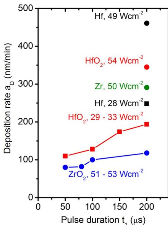
**Figure 1:** The figure illustrates very high deposition rates reached during reactive HiPIMS of  $ZrO_2$  and  $HfO_2$  thin films. All films were highly optically transparent (value of an extinction coefficient at the wavelength of 550 nm,  $k_{550}$ , below 0.001 for all films) and densified (mass density reached bulk mass density).
