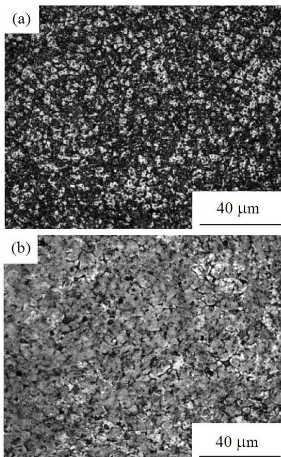
**Figure 1:** Morphology of steel surface after PEN/C (a) and PEP for 60 s (b).
