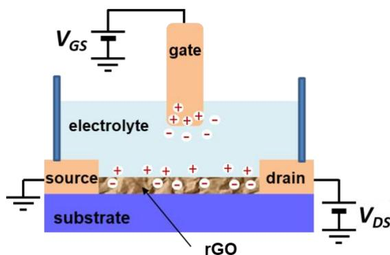
**Figure 1:** Scheme of the GFET setup in the electrolyte-gated configuration (EGFET). The channel is made of rGO obtained from the *in situ* electro-reduction of inkjet printed GO.
