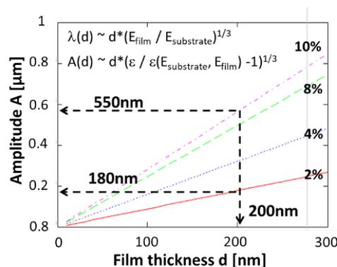
**Figure 1:** Wrinkle amplitude  $A$  as a function of pre-strain (2-10%) for a-C:H films ( $d = 200$  nm) on TPU substrate.
