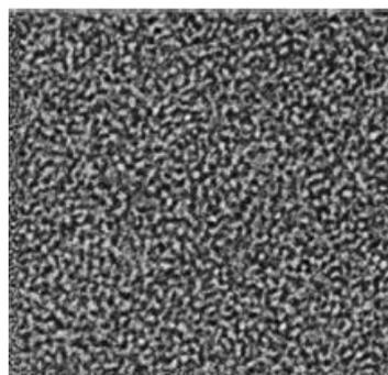
**Figure 1:** Figure illustrating the nanophase separation of phosphonium cation combined with phosphate anion with a content of 10 phr from the DGEBA based epoxy network [4]
