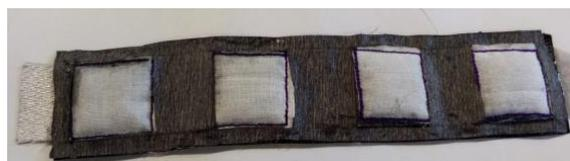
**Figure 2:** Prototype of a multi-cell flexible textile Al-Air battery with cells arranged on a plane.
