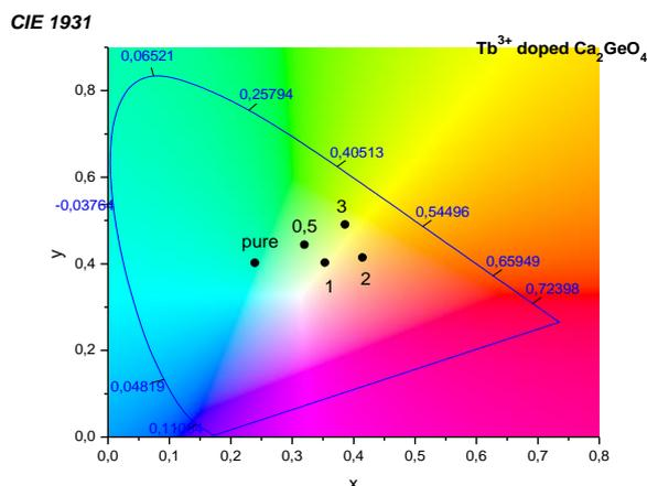
**Figure 1:** CIE coordinates of the  $\text{Tb}^{3+}$  doped  $\text{Ca}_2\text{GeO}_4$  samples with different concentrations of the active ion, illustrating the possibilities to tune colors by changing dopant concentration.
