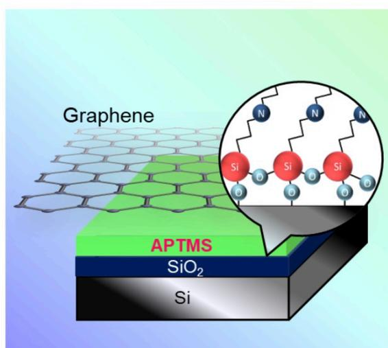
**Figure 1:** Schematic drawing of graphene on an APTMS-treated  $SiO_2/Si$  substrate. APTMS molecules are densely packed on the  $SiO_2/Si$  substrate. Inset: the Si atom (red) at the head-group of the APTMS molecule covalently bonds to an oxygen atom (light blue) of the silanol group on the  $SiO_2/Si$  substrate.
