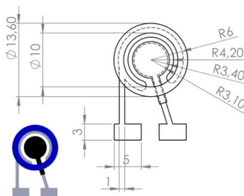
**Figure 1:** Printed electrolysis cell design. Working electrode (black), counter electrode (grey) and hydrophobic plastic ring (blue).
