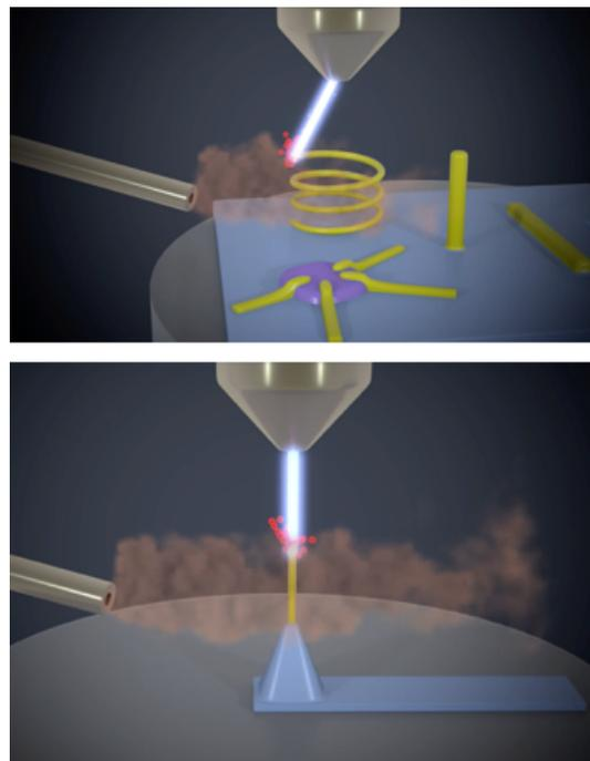
**Figure 1:** Figure illustrating the growth of nanostructures by FEBID and FIBID
