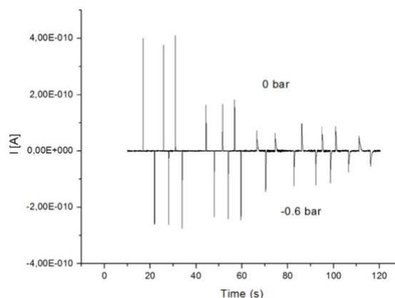
**Figure 1:** Current flowing through Schottky diode contact under cyclic pressure application ( $p=0,6$  Bar)
