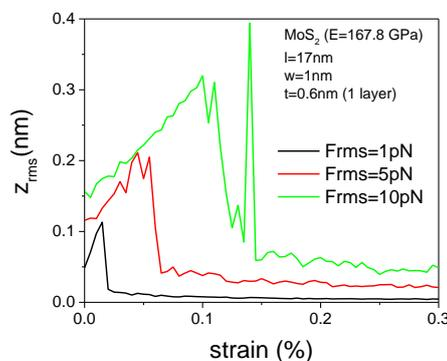
**Figure 2:** Dynamic response of figure 1 ribbon for different excitation intensities.
