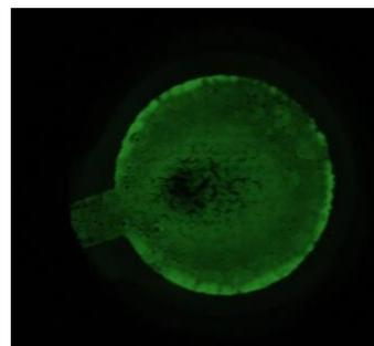
**Figure 2:** Tb(III) chelate label HECL emission under excitation by cathodic voltage pulses at ethyl cellulose-carbon black electrode. Conditions: pulse voltage  $-46$  V, pulse charge  $31.5 \mu\text{C}$ , frequency  $50$  Hz,  $0.01$  M  $\text{NaN}_3$  in  $0.05$  M  $\text{Na}_2\text{B}_4\text{O}_7$ ,  $0.1$  M  $\text{Na}_2\text{SO}_4$ .
