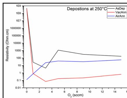
**Figure 1:** Resistivity as function of O<sub>2</sub> flow rates for the as-deposited, vacuum- annealed and air-annealed samples.
