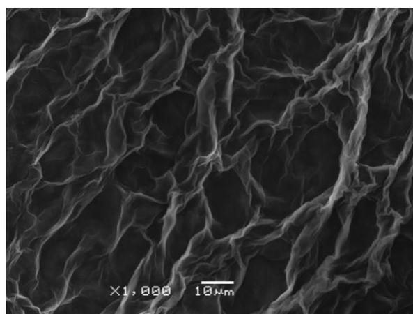
**Figure 1.** The drawing illustrates layers of graphene oxide film (1 % aqueous emulsion)
