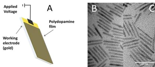
**Figure 1:** Figure A) showing the schematic procedure for polydopamine electropolymerization B) TEM image of NRs and C) TEM image of NRs embedded in polydopamine freestanding film.
