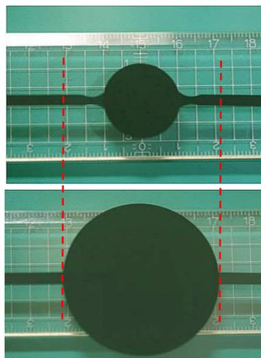
**Figure 1:** Expanding Circular Actuator up to 630%
