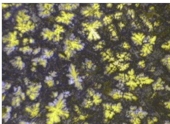
**Figure 1:** Figure illustrating the dendritic morphology of high-entropy AlCrFeCoNi<sub>1.4</sub> alloy after electrochemical etching in oxalic acid 10% for one minute.
