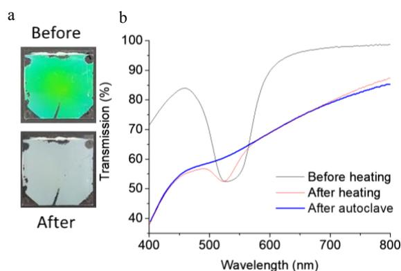
**Figure 2:** Supramolecular Humidity Temperature Time Integrator as a steam sterilization sensor. a: Sensor before and after steam sterilization procedure. b: UV-VIS spectrum comparing only heating the coating to the spectrum after steam sterilization to illustrate the contribution of humidity to the scattering effect.
