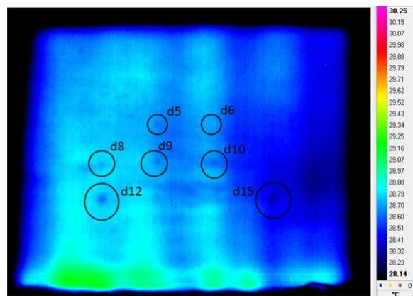
**Figure 1:** Geometry of the panel containing artificial defects and an example of the thermal map obtained during experimental measurements.
