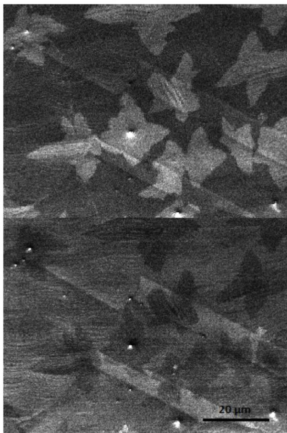
**Figure 1:** The use of low energy electrons for the determination of the number of graphene layers. Few-layer graphene flakes on Cu foil observed at 7.2 eV (upper) and 12.3 eV and their reflectivity changes caused by different landing energy of the electron beam.
