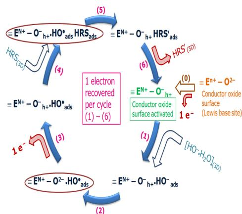
**Figure 1:** Principal steps of an electrocatalytic reaction cycle explaining the hydroxyl radical generation and the recovering of elementary electric charges from water by a conductor oxide surface.
