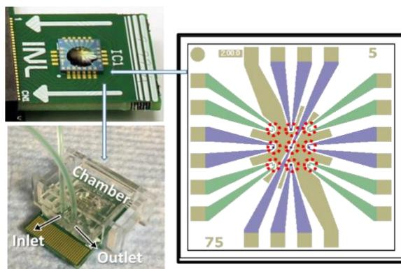
**Figure 1:** (counterclockwise from right to left) The sensor chip containing 9 GFETs (highlighted in red) is wire bonded to a PCB that is inserted in the control board. A PDMS flow cell, fitting the sensor layout, can be assembled to the chip prior to insertion in the board.
