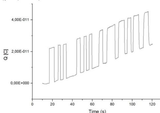
**Figure 2:** Charge changes on the Schottky contact under cyclic pressure application ( $V=0$  V)
