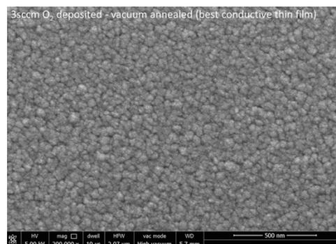
**Figure 2:** SEM images for the best conductive sample before and after annealing.
