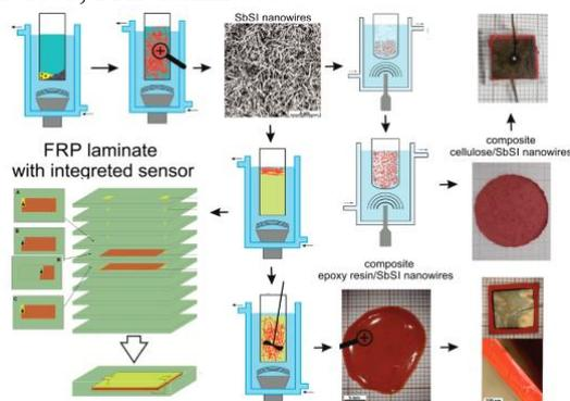
**Figure 1.** Scheme of sonochemical preparation of: SbSI nanowires, the epoxy resin/ SbSI nanowire and cellulose/SbSI nanowires composites, generator/sensor assembly and scheme of FRP laminate with integrated sensor.
